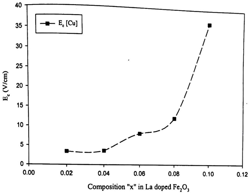
Fig.4.3 Composition dependence of the coercive field of La doped  $Fe_2O_3$  thin film device.
