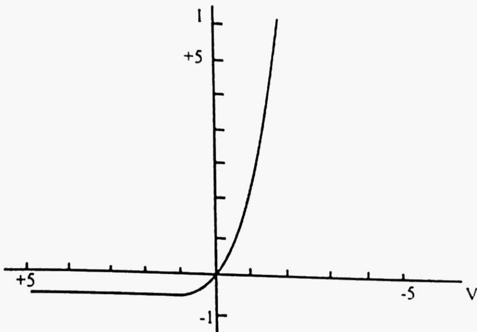
Fig 3.6 (c) Ideal diode current-voltage characteristic.
