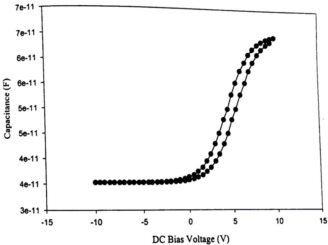
Fig. 4.6(a) Capacitance -Voltage characteristics of the La doped  $\text{Fe}_2\text{O}_3$  ( $x = 0.02$ ) thin film device formed by annealing at  $600^\circ\text{C}$ .
