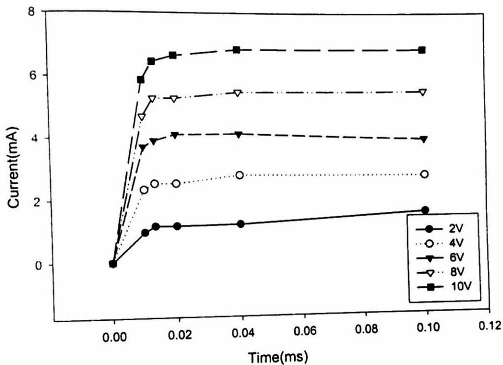
Fig. 4.14(b) Transient current - time curve measured with La doped Fe<sub>2</sub>O<sub>3</sub> (x=0.04) thin film capacitor (formed at 600°C) for Cu electrode.
