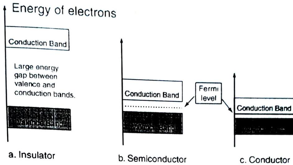
Fig. 2.4 Energy band diagrams (a) Insulator (b) Semiconductor and (c) Conductor.
