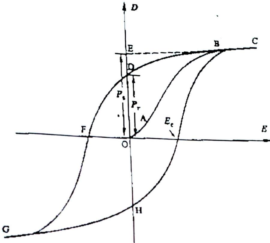
Fig 1.1 A Typical P-E Hysteresis Curve.
