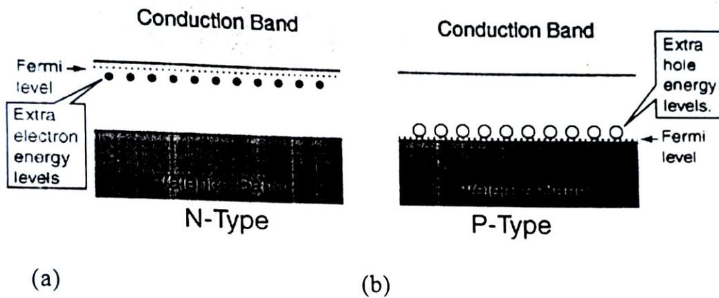
Fig. 2.3 Energy band diagram of extrinsic semiconductor showing (a) the donor level and (b) the acceptor level.
