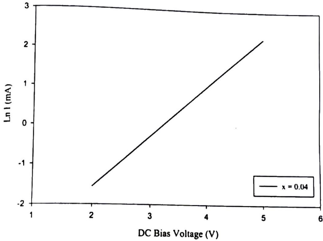
Fig.4.11(b)  $\ln I$  vs.  $V$  characteristics of La doped  $\text{Fe}_2\text{O}_3$  thin film device ( $x = 0.04$ ) formed at  $600^\circ\text{C}$ .
