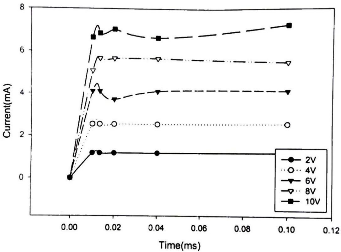
Fig. 4.14 (e) Transient current - time curve measured with La doped Fe<sub>2</sub>O<sub>3</sub> (x=0.10) thin film capacitor ( formed at 600<sup>o</sup>C) for Cu electrode.
