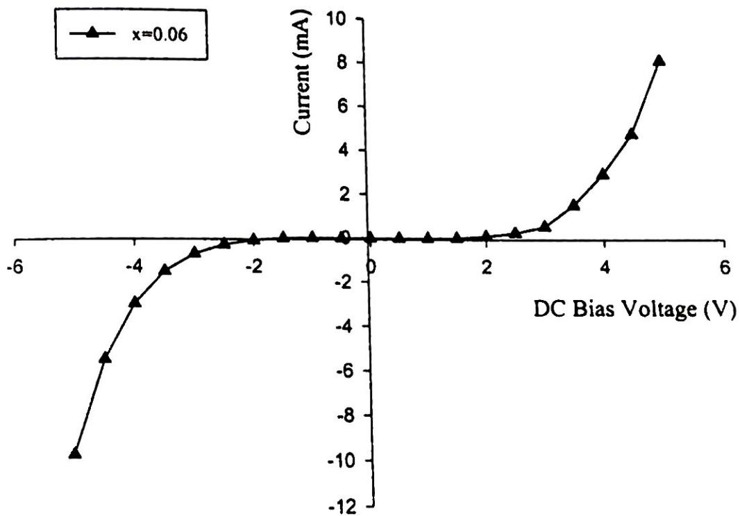
Fig.4.10(c) I-V characteristics of La doped Fe<sub>2</sub>O<sub>3</sub> thin film
