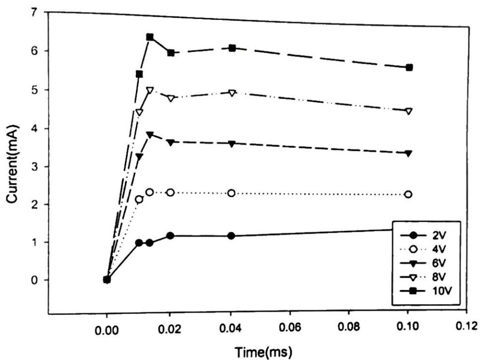
Fig.4.14 (d) Transient current - time curve measured with La doped Fe<sub>2</sub>O<sub>3</sub> (x=0.08) thin film capacitor (formed at 600°C) for Cu electrode.
