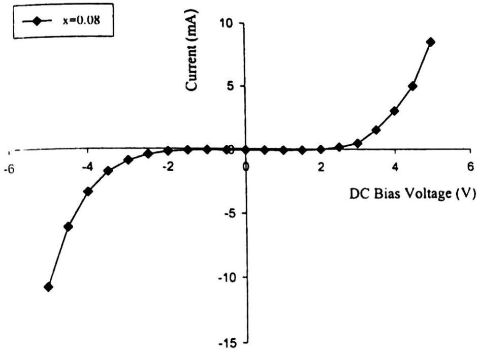
Fig.4.10 (d) I-V characteristics of La doped Fe<sub>2</sub>O<sub>3</sub> thin film (x = 0.08) formed at 600°C
