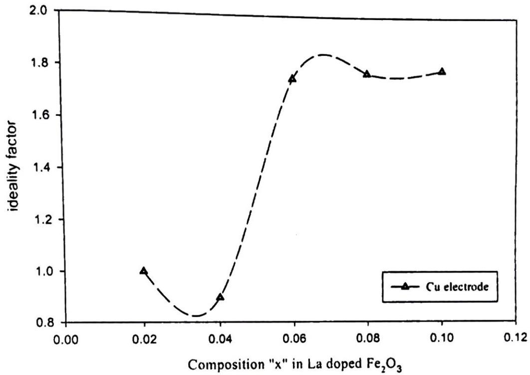
Fig.4.13 Composition dependence of the ideality factor of La doped Fe<sub>2</sub>O<sub>3</sub> thin film device.
