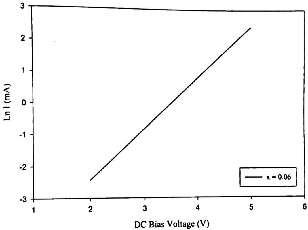
Fig.4.11(c) Ln I vs. V characteristics of La doped  $\text{Fe}_2\text{O}_3$  thin film device ( $x = 0.06$ ) formed at  $600^\circ\text{C}$ .
