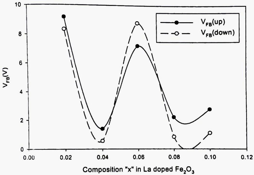
Fig. 4.8 Composition dependence of the flat band voltage of La doped  $Fe_2O_3$  thin film capacitor.
