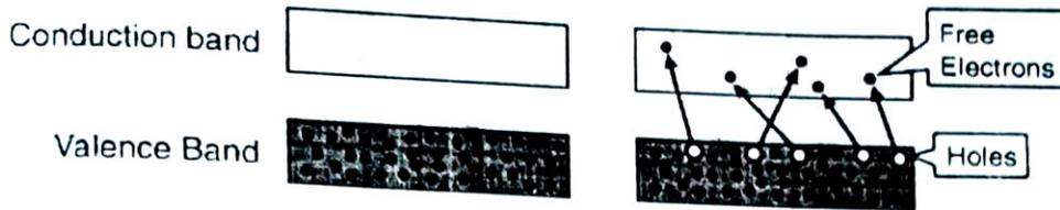
Fig. 2.2 Energy band diagram of an intrinsic semiconductor
