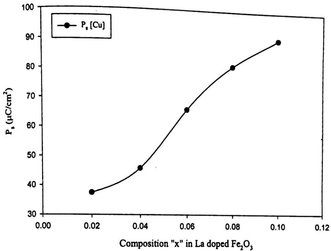
Fig.4.4 Composition dependence of the spontaneous polarization of La doped  $\text{Fe}_2\text{O}_3$  thin film device.
