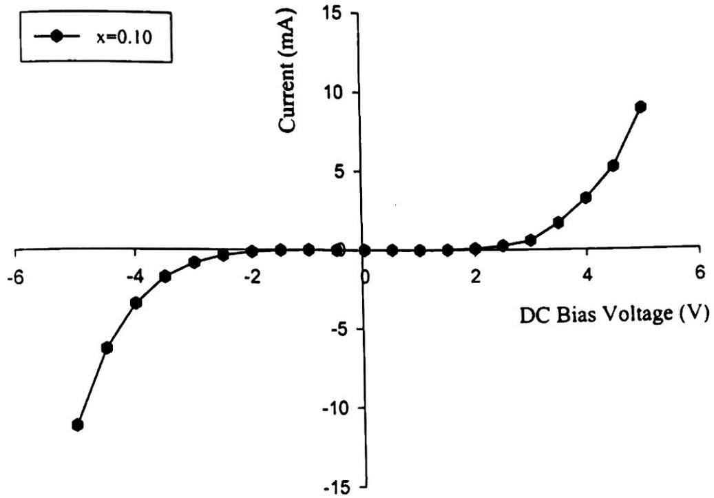
Fig.4.10(e) I-V characteristics of La doped Fe<sub>2</sub>O<sub>3</sub> thin film
