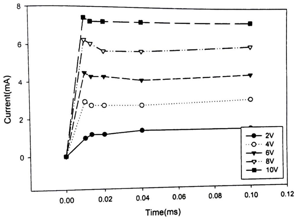
Fig. 4.14(c) Transient current - time curve measured with La doped  $\text{Fe}_2\text{O}_3$  ( $x=0.06$ ) thin film capacitor (formed at  $600^\circ\text{C}$ ) for Cu electrode.
