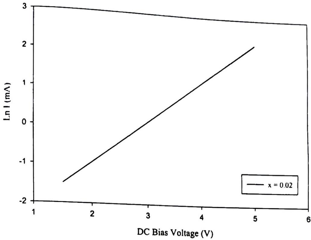
Fig.4.11(a)  $\ln I$  vs.  $V$  characteristics of La doped  $\text{Fe}_2\text{O}_3$  thin film device ( $x = 0.02$ ) formed at  $600^\circ\text{C}$ .
