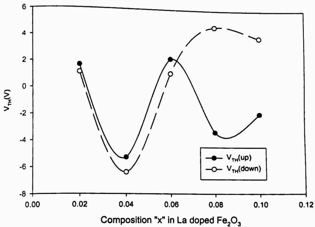
Fig .4.7 Composition dependence of the Threshold voltage of La doped  $Fe_2O_3$  thin film capacitor.
