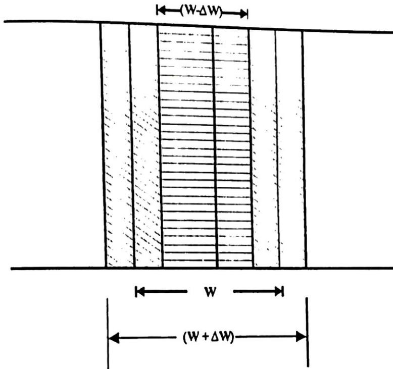
Fig 3.5 Change in the depletion region width caused by an increment  $\Delta V_a$  in the junction bias.
