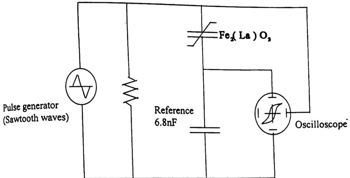
Fig 3.3 Measurement of Polarization with Sawyer - Tower Circuit.
