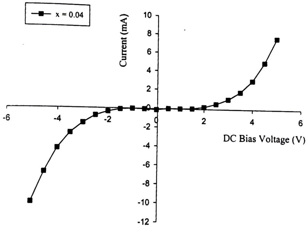
Fig.4.11(b) Ln I vs. V Characteristics of La doped Fe<sub>2</sub>O<sub>3</sub>
