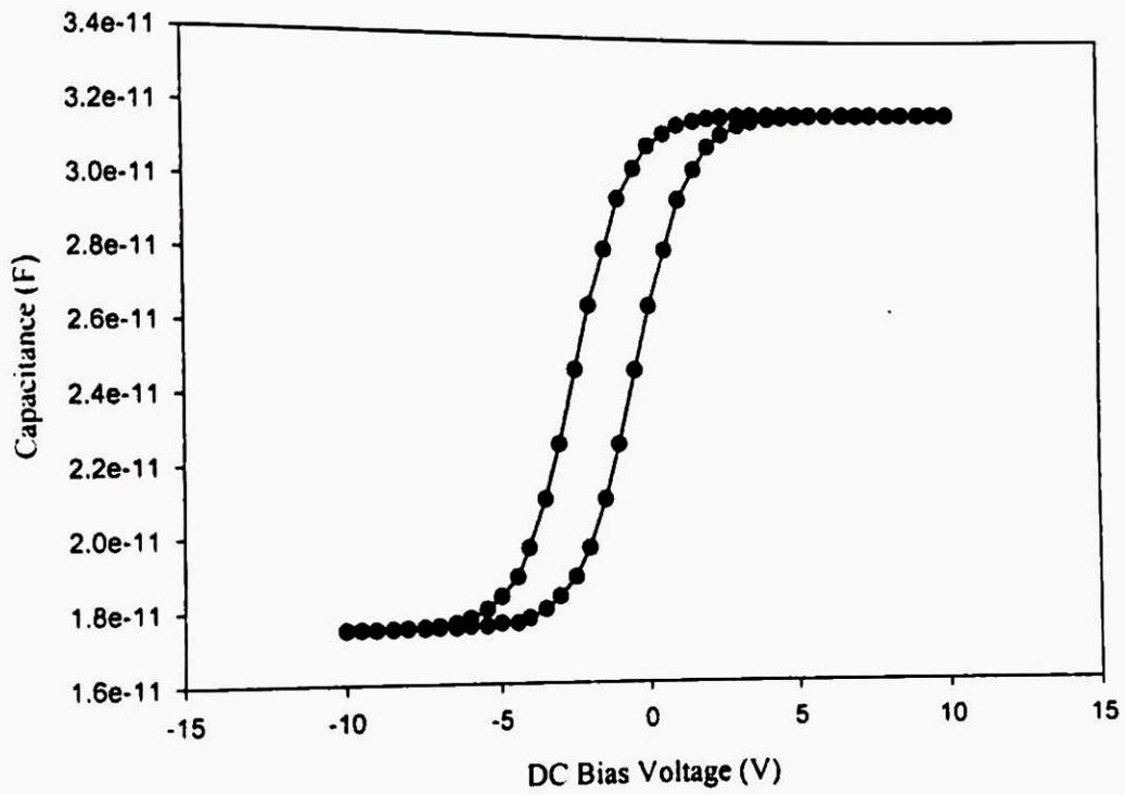
Fig.4.6(d) Capacitance -Voltage characteristics of the La doped  $\text{Fe}_2\text{O}_3$  ( $x=0.08$ ) thin film device formed by annealing at  $600^\circ\text{C}$ .
