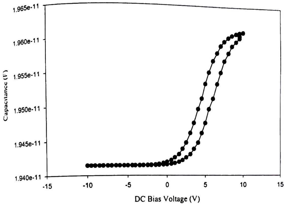
Fig.4.6(c) Capacitance -Voltage characteristics of the La doped  $\text{Fe}_2\text{O}_3$  ( $x=0.06$ ) thin film device formed by annealing at  $600^\circ\text{C}$ .
