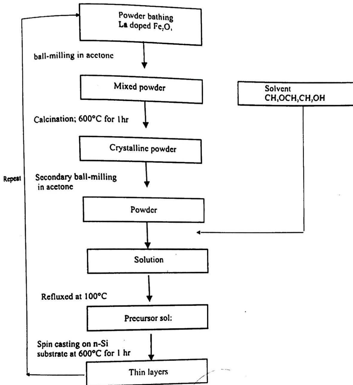
Fig 3.2 Flow diagram for fabrication of  $(1-x)\text{Fe}_2\text{O}_3 + (x)\text{La}_2\text{O}_3$  thin layers.
