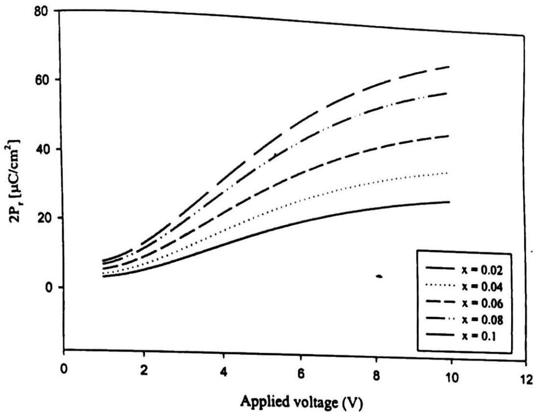
Fig.4.2 Saturation properties of remanent polarization of La doped  $\text{Fe}_2\text{O}_3$  thin films device with Cu electrode.
