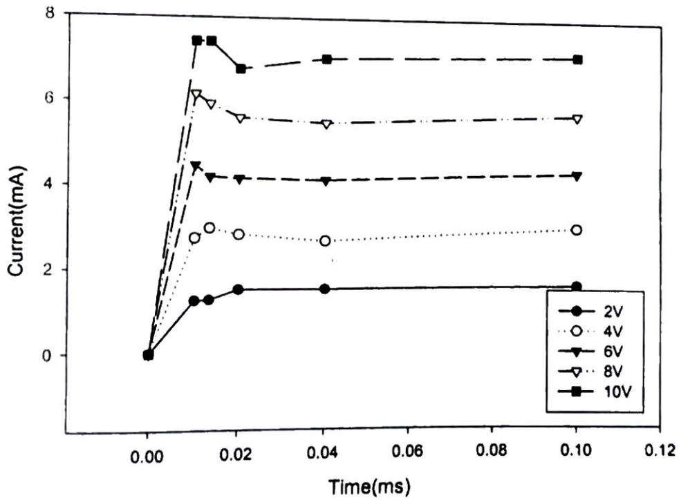
Fig. 4.14 (a) Transient current - time curve measured with La doped Fe<sub>2</sub>O<sub>3</sub> (x=0.02) thin film capacitor (formed at 600<sup>o</sup>C) for Cu electrode.
