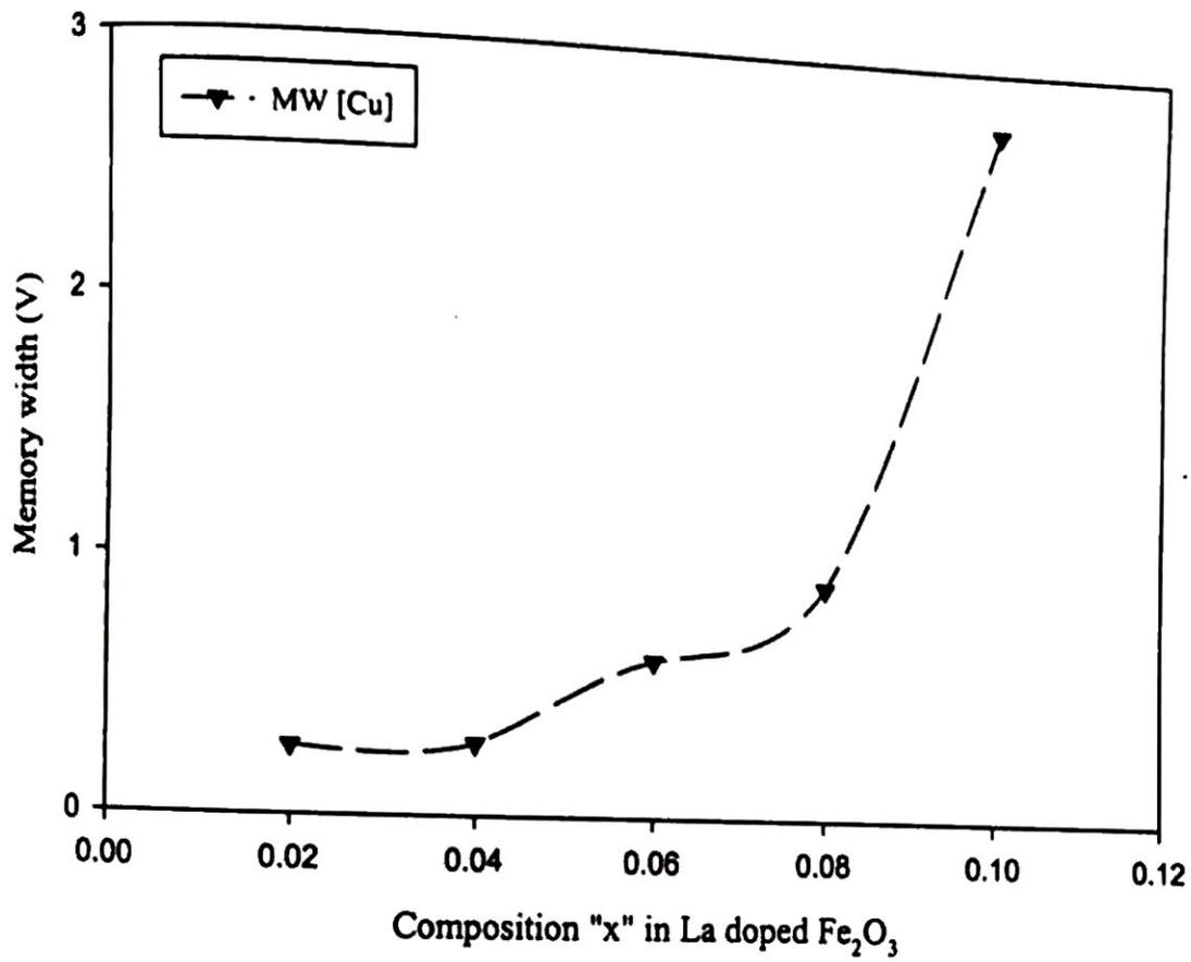
Fig.4.5 Composition dependence of the memory width of La doped Fe<sub>2</sub>O<sub>3</sub> thin film device.
