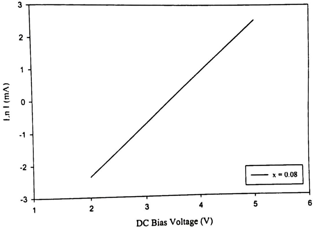
Fig.4.11(d) Ln I vs. V characteristics of La doped  $\text{Fe}_2\text{O}_3$  thin film device ( $x = 0.08$ ) formed at  $600^\circ\text{C}$ .
