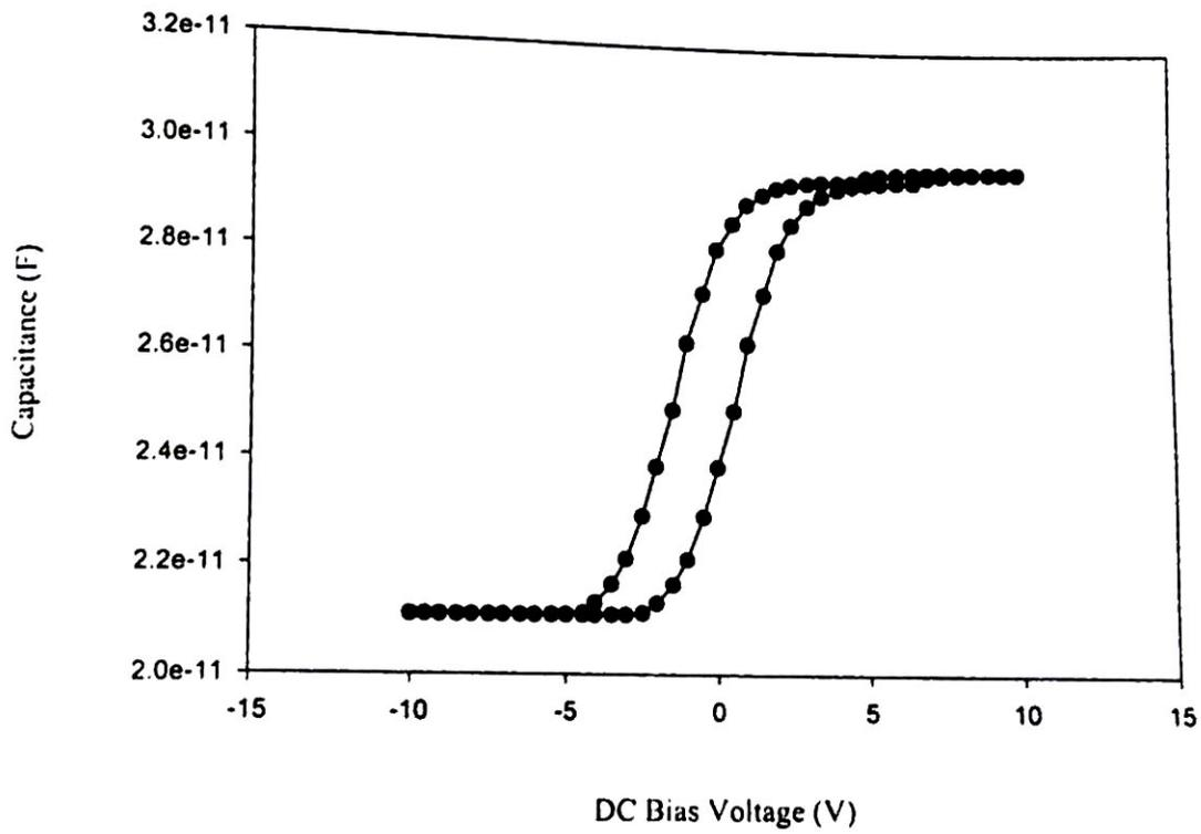
Fig.4.6(e) Capacitance -Voltage characteristics of the La doped  $\text{Fe}_2\text{O}_3$  ( $x = 0.10$ ) thin film device formed by annealing at  $600^\circ\text{C}$ .
