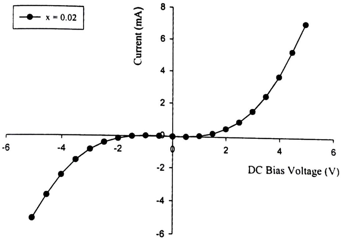
Fig.4.10(a) I-V characteristics of La doped Fe<sub>2</sub>O<sub>3</sub> thin film
