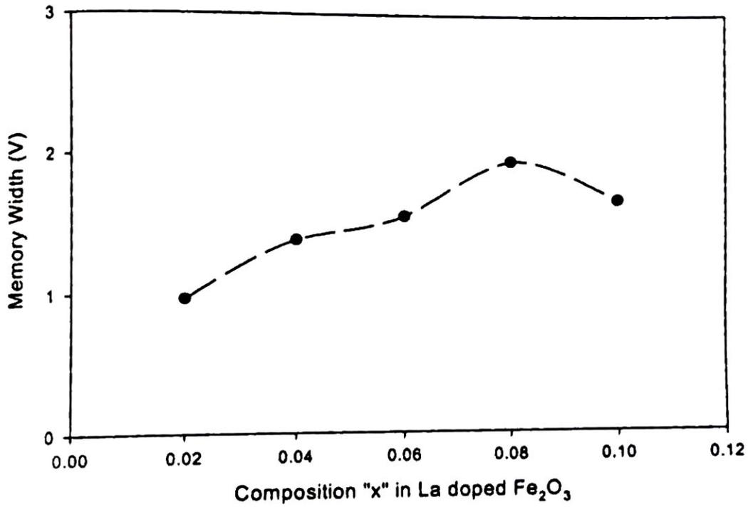
Fig.4.9 Composition dependence of the memory width of La doped Fe<sub>2</sub>O<sub>3</sub> thin film capacitor.
