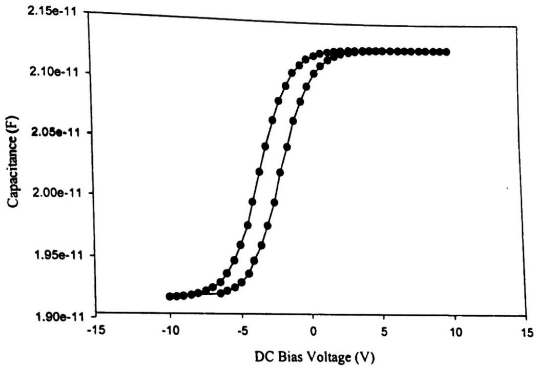
Fig.4.6(b) Capacitance -Voltage characteristics the La doped  $\text{Fe}_2\text{O}_3$  ( $x=0.04$ ) thin film device formed by annealing at  $600^\circ\text{C}$ .
