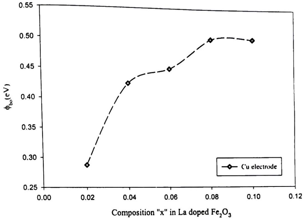
Fig.4.12 Composition dependence of the zero-bias barrier height of La doped  $Fe_2O_3$  thin film device.
