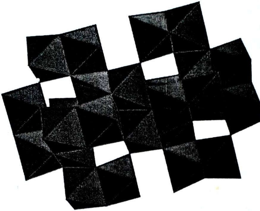
Fig. 2.6 The crystal structure of  $\text{Fe}_2\text{O}_3$ .
