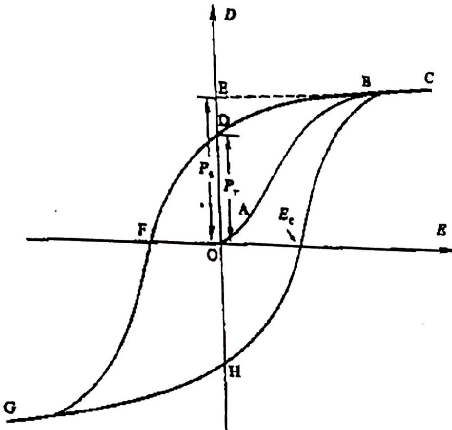
Fig 3.4 A Typical P-E Hysteresis Loop observed with Ferroelectric sample.
